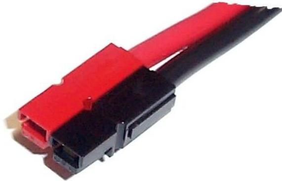
The housings should be mated according to the picture at left, viewing from the contact side (opposite the wire side), tongue down, hood up, RED on the LEFT, and BLACK on the RIGHT.
