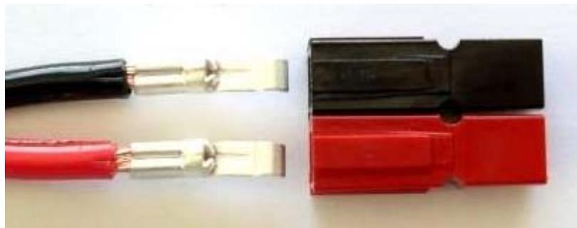
Tug slightly on the assembled connector to make sure the contacts are locked in place. If you have trouble getting the contact to lock into the housing you may have squashed the contact wider and deformed it. Also look at the side profile of the contacts before and after crimping. You may have to bend it back straight before inserting it in to the housing.
